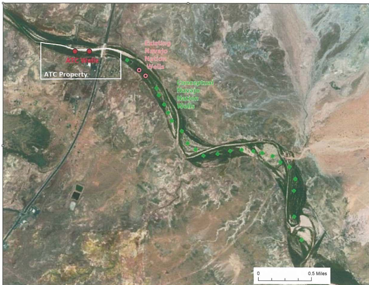
Figure 8. Example Navajo Nation wellfield layout for Scenario 4.
